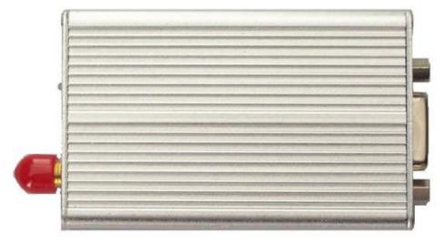
LS-U1000D is a low power wireless transceiver data module. With metal shell, DB9 Connector and good stability, reliability, it is widely used for kinds of outdoor wireless applications, such as remote control, industry automation, wireless telemetry and so on. This module can be connected with micro-controller, PC, RS485 equipments and other devices with UART port directly.
